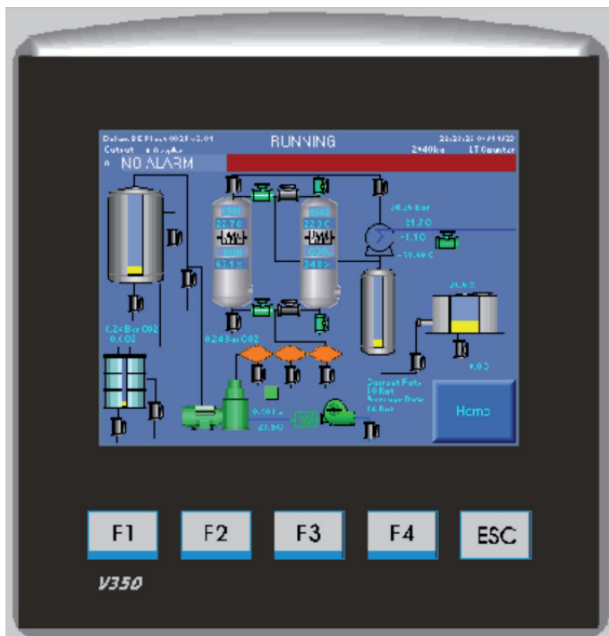
CO 2 recovery process, flow chart
