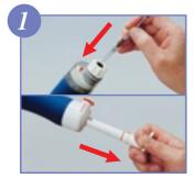
Insert <u>a sealed, unbroken detector</u> <u>tube</u> into the rubber tube connector. Align the red line on the bottom case and that of shaft, and pull the handle to full stroke locked position.
