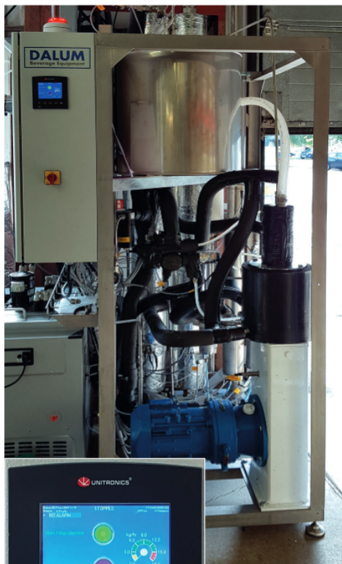
Dalum's skid-mounted CO 2 recovery unit in-situ at Gadd's Ramsgate Brewery with (inset) integrated controller
