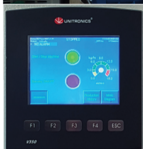
Dalum's skid-mounted CO 2 recovery unit in-situ at Gadd's Ramsgate Brewery with (inset) integrated controller
